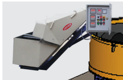
3-bin Hydraulic Hopper with weight batching system
